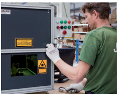
Laser beam during logo engraving process (II).
