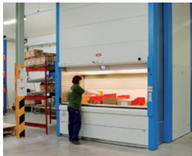
Kardex: automated high-capacity storage system.
